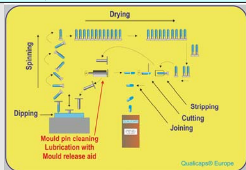
Figure 1. Diagram of hard capsule manufacturing machine to show machine sequence and where point mould lubricant is applied.
