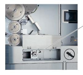
Printing position adjust knob (Adjusting the direction of travel)
