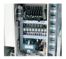
**8** The control panel is contained in the main unit.
