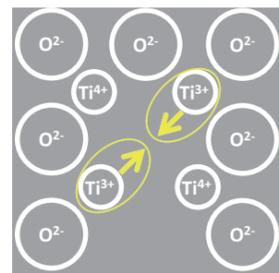
The removal of oxygen atom causes change of ratio of titanium atom to oxygen atom. This change of ratio induces the color change of titanium dioxide from white to grey.
