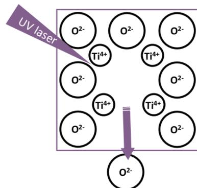
The ratio of titanium dioxide(Ti) to oxygen(O) in titanium dioxide is 1:2. UV laser is irradiated on the titanium dioxide then oxygen atom is removed.
