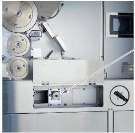
Printing position adjust knob (Adjusting the direction of travel)
