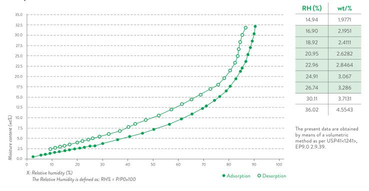
Quali-V® Extra Dry capsules maintain their physical stability and show minimal brittleness when exposed to ambient conditions with low humidity.
