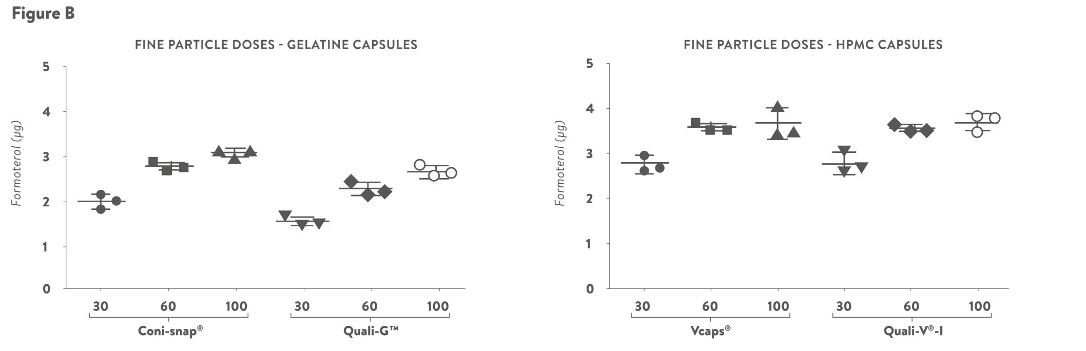
Figure B. FPD (µg) determined using the NGI (30 L/min 8 s, 60 L/min 4 s, 100L/min 2.4 s, n=3) connected to the Axahaler®, filled successively with 10 capsules pre-filled and pre-stored.
