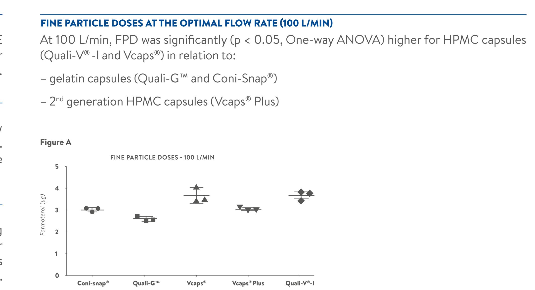
Figure A. FPD (µg) determined using the NGI (100L/min 2.4 s, n = 3) connected to the Axahaler<sup>®</sup>, filled successively with 10 capsules pre-filled and pre-stored.
