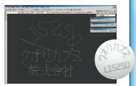
Marking letters, mark or logo can be made by CAD which allows flexible design. Test printing and printing result check are not needed before production.
