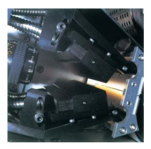
**Rear surface inspection (100% coverage)** After alignment (rotation from vertical to horizontal orientation), the unimprinted tablets are held by suction inside pockets in the inspection roller and illuminated with a uniform light source while a 5,150-element CCD line sensor camera inspects their rear surfaces.
